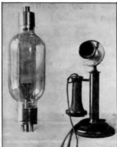
1 K.W. Tube Compared to Ordinary Desk Telephone
